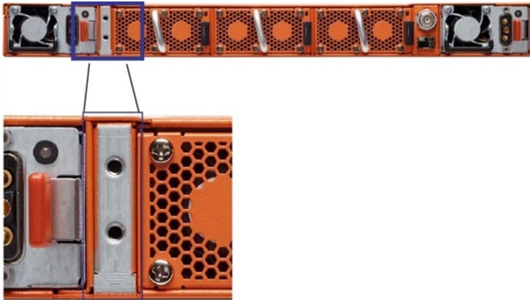
Figure 1 Holes for Ground Screws (DC-Powered GigaVUE-HC1)
